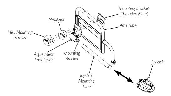
FIGURE 9.2 Repositioning the Joystick
